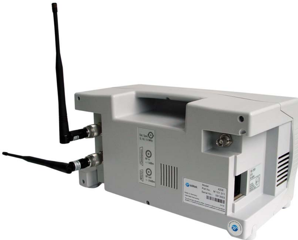
Figure 3: The back of the 4208 shows separate connectors for radio frequency input and output. Isolation between receive and transmit paths can be improved by arranging the two antennas in a 90° angle.
